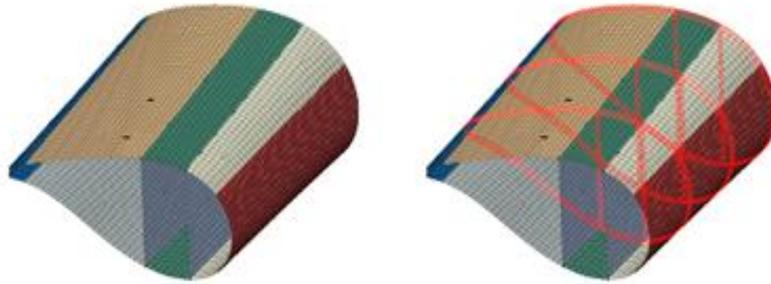
*Figure 3.19 Finite element shell model in BECAS [14]*
